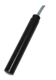
The OxyGuard Mini Probe is a membrane covered galvanic cell that generates an electrical signal proportional to the oxygen pressure it senses. It is a small version of the probe that has become the preferred choice of dissolved oxygen probe for fish farmers all over the world.
